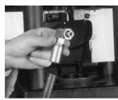
SELECT proper size collet (referenced in the Crimp Specifications Manual) for hose type and size being crimped. INSERT collet halves into adapter ring. PLACE proper size hose end on hose. Be sure to bottom the hose.
