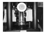
assembly through the bottom of the base adapter ring and between the two collet assembly halves. To achieve a full flat crimp for 4SP/6SP fittings, locate the bottom of the socket approximately 1/8" (3mm) from the bottom edge of the collet halves as referenced in Eaton Crimp Specifications.
