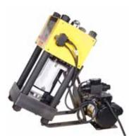
IT IS RECOMMENDED THAT THE PUMP BE ON AN INDIVIDUAL 20 AMP SERVICE OUTLET.
