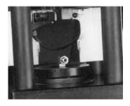
3. SELECT PROPER spacer ring referenced in the Crimp Specifications Manual. INSERT hose assembly from below, between collet halves.
