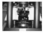
1. OPEN the pusher halves. NOTE: Lubricate the inside cone of the base adapter ring and external surfaces of the collet assembly with a high-efficiency PTFE based lubricant (T-400-G).
