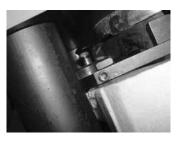
PULL the pusher tab upward. The pusher tab is located behind the top of the pushers at the back of the machine.
