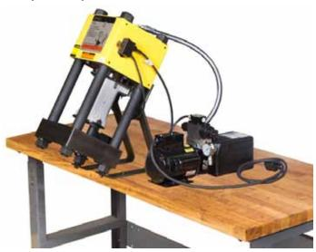
**Note**: Machine to be mounted on sturdy surface to accommodate the machine and components (500+lbs.).
