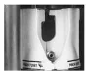
4. CLOSE pusher halves. HOLD SWITCH ON. When spacer ring (shown in step 3 in black) bottoms on adapter ring below it, the crimp is complete.
