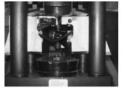
7. SELECT the proper collet assembly for hose type being crimped as referenced in the Crimp Specifications Manual or chart and insert the collet assembly into the base adapter ring.
